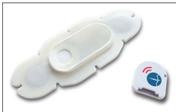
Figure 1. Multisensor monitoring device consisting of a disposable sensor patch with a disposable battery and a reusable sensor electronics module.
