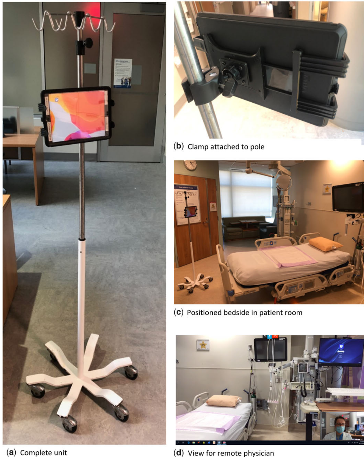
Figure 3. Tele-ICU (iPad on a stick): rapidly deployed mobile virtual consult service. (A) The complete unit; (B) clamp attached to pole; (C) positioned bedside in patient room; (D) view for remote physician.
